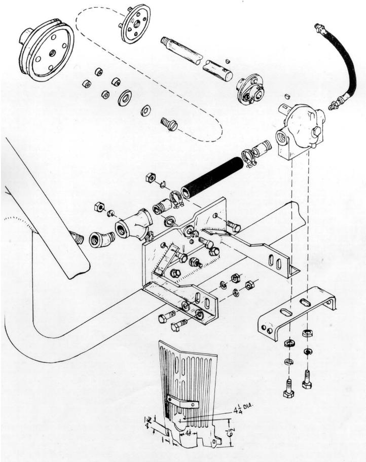
Figure 3, Front Installation, Ford Model 8N and 9N
